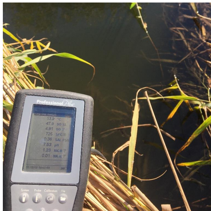
Figure 1 Regularly checking oxygen levels will help identify underlying problems at an early stage – in this example we found a dissolved oxygen level of just 47%. This confirmed the oxygen levels in the watercourse were dropping and aeration equipment was put in to help save fish
