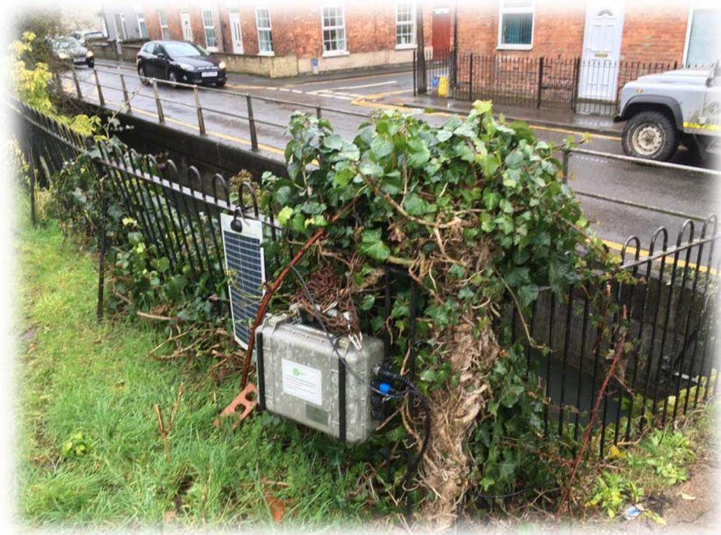
*Figure 2 Solar powered data logger*
